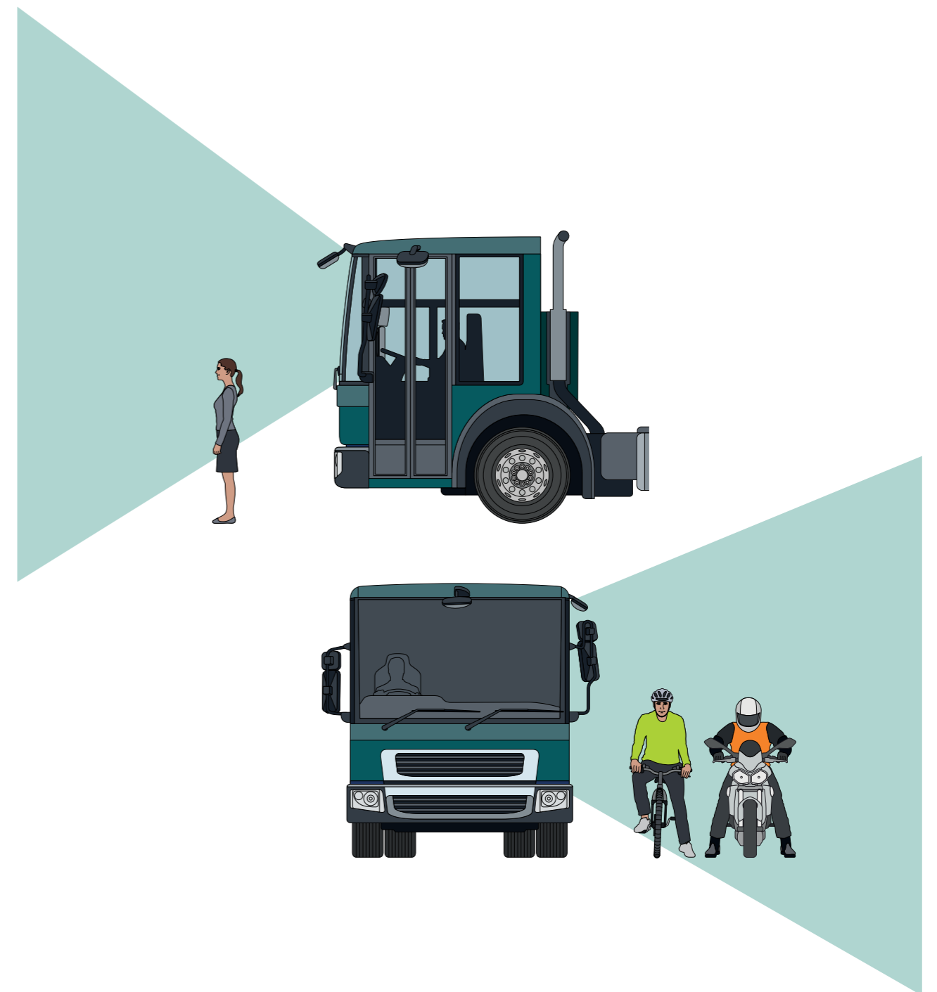
Figure 14: High vision HGVs increase drivers' ability to see other road users directly through their cab windows
