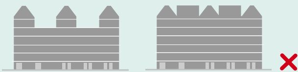
Roof with irregular cornice line and varied pitches
