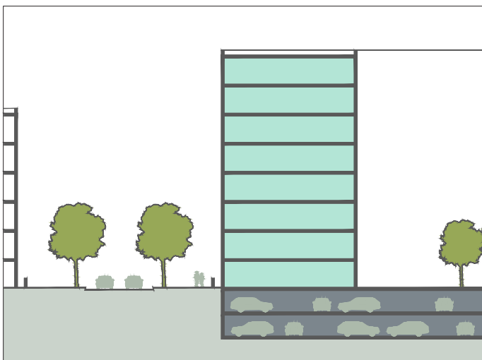
High density: basement parking
